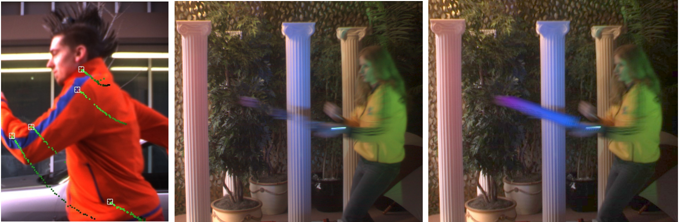
Figure 1: Motion and incident illumination capture in a natural setting with imperceptible marker tags. (Left) Traces of hidden tags superimposed on an actor running in sunlight. (Middle) A video frame from a recording session. (Right) A virtual sword inserted with matching location, orientation, lighting and motion blur.
